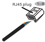
Figure 3.27 Strip the insulation layer and connect to RJ45 plug
