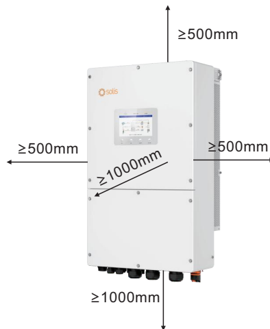
Figure 3.5 Inverter Mounting Clearances
