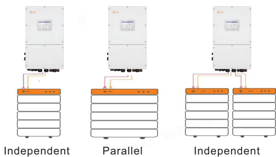
Figure 3.20 Battery connection types
