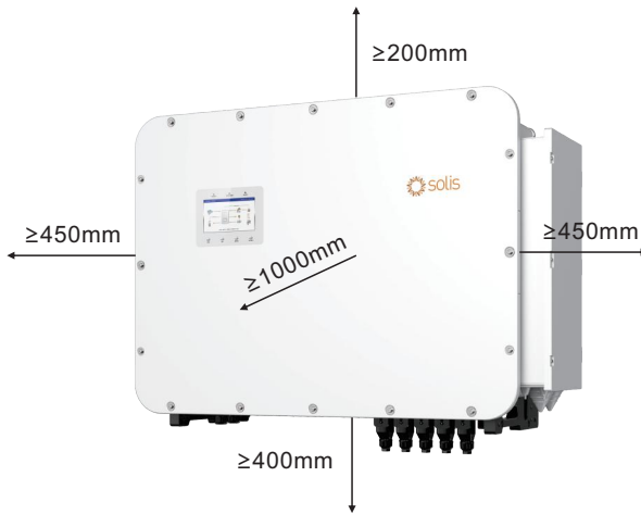
Figure 3.5 Inverter Mounting Clearances
