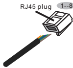
Figure 3.39 Strip the insulation layer and connect to RJ45 plug
