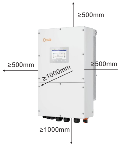
Figure 3.5 Inverter Mounting Clearances
