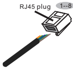
Figure 3.21 Strip the insulation layer and connect to RJ45 plug
